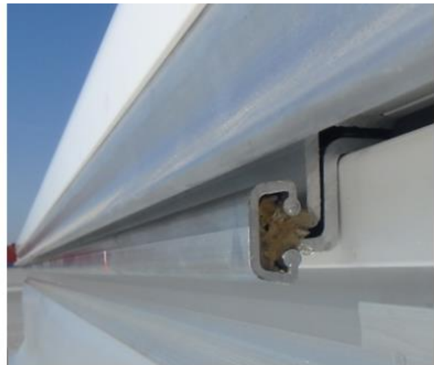
Fig. 20. Hinge with fitted connector.
